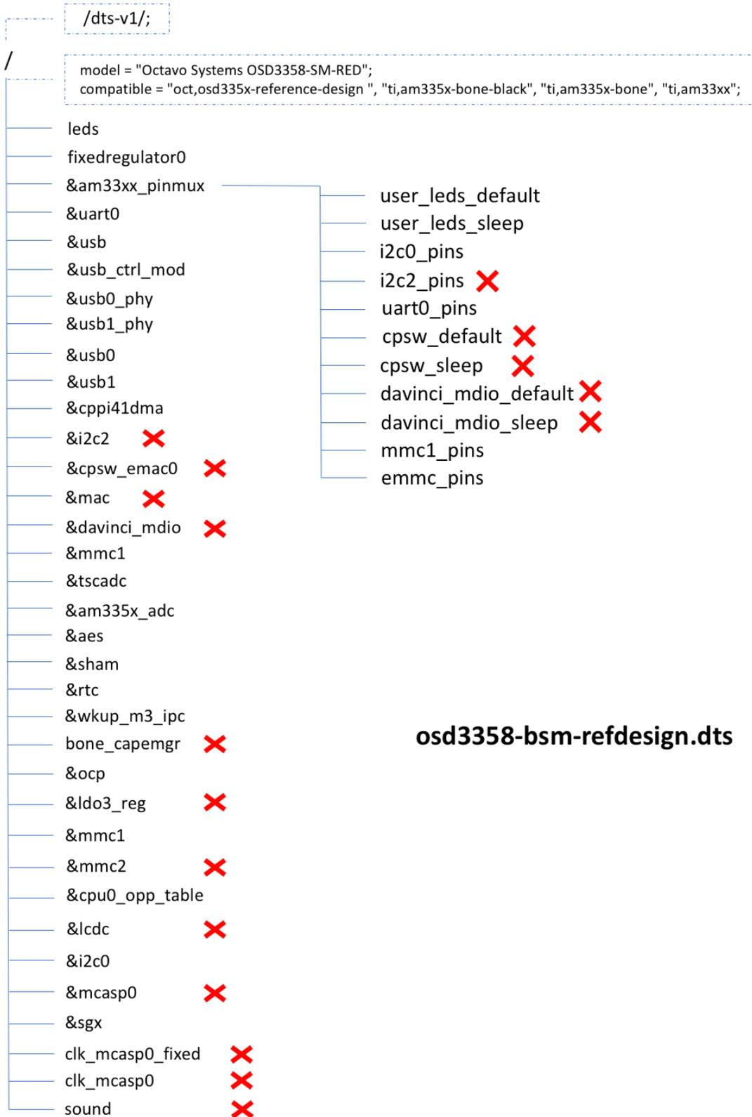
Figure 3 osd3358-bsm-refdesign.dts before modifications
