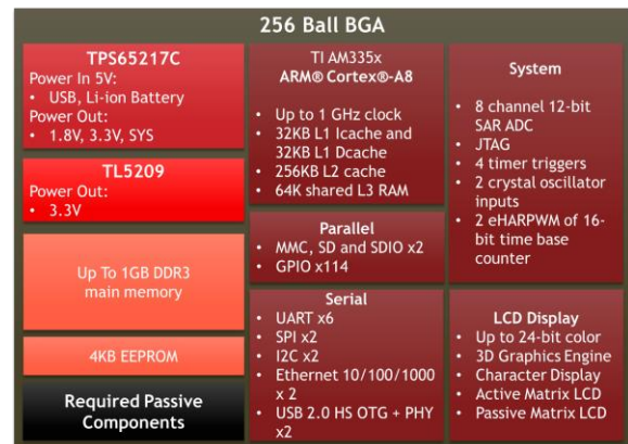
Figure 1. OSD335x-SM Block Diagram
