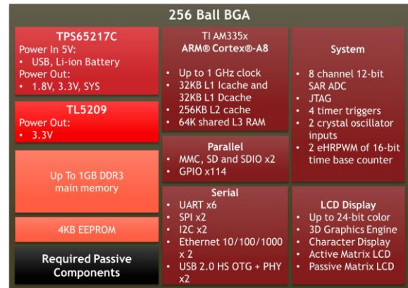
Figure 1. OSD335x-SM Block Diagram
